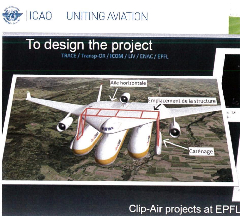
Figure 14 : architecture Clip-Air
