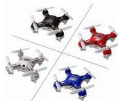
Figure 4.2.4.6.2: micro-UAV with electric propulsion
