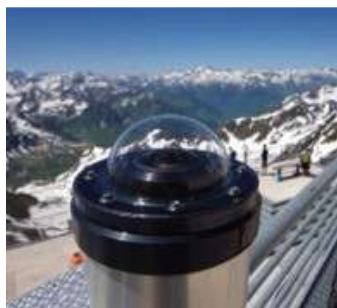
Figure 6.3.2.4 - Multiple Fisheye cameras (hemispherical wide-angle vision) of the FRIPON network allow global coverage of the territory.
