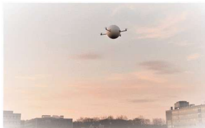
Figure 5.12.3.4.4.2.1 - Spherical UAV with external motorization
