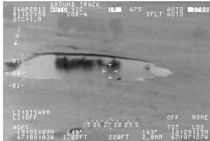
Figure 4.2.4.3.1 – IR image of the object with contrast inversion of the IR landscape background (local image processing effect). The object is to the right and at the base of the sighting cross
