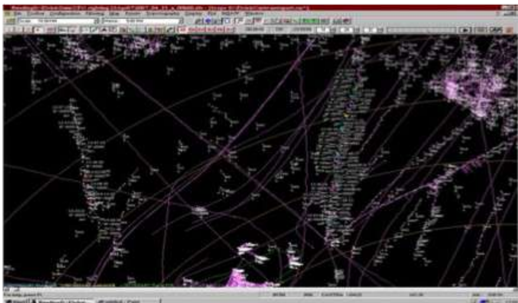
Figure 6.2.5 : example of visualization of a primary civilian radar situation (echoes are visible) - Jersey ATC radar
