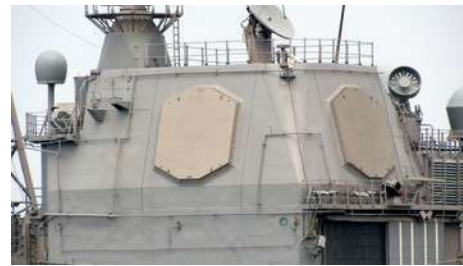
Figure 6.2.4 : example of a naval air defense Multifunction radar similar to the radar used in the US Nimitz case (2004) to track UAP
