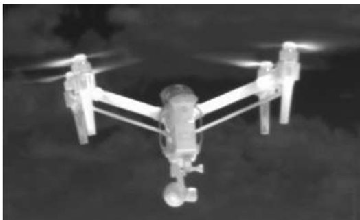
Figure 5.2.1.1 : thermal image of micro drone in band 2 (gray body type emission)
