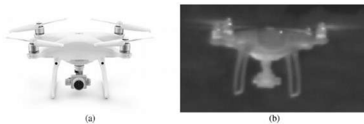
Fig. 1 (a) UAV1 DJI Phantom Pro 4 model and (b) MW image.
